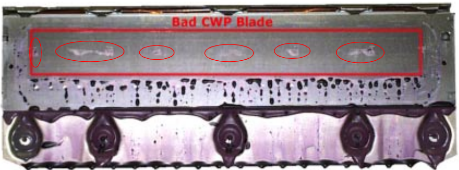
Fig 3-3 Faceplate showing streaks and smudges from a poor wipe
