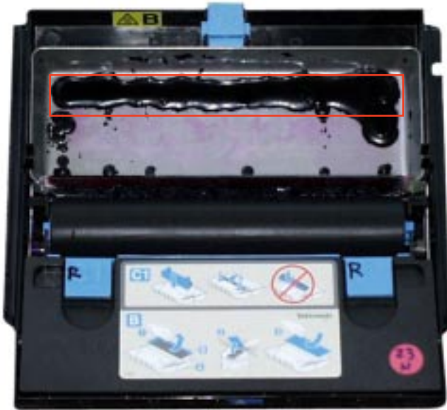
Fig 3-5 Maintenance tray showing good purge
