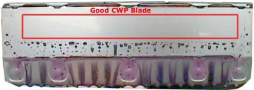
Fig 3-2 Faceplate showing blade wipe with no drops, smudges or streaks
