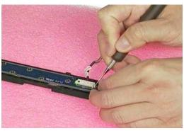
5. Remove 7 screws (M2\*3L(K)) and take the switch board away.
