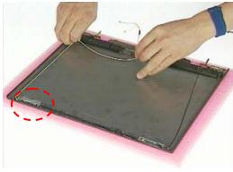
TOP CASE MODULE 8. Reomve the speaker cable, then remove 1screw(M2\*3L(K)) and 1 screw on the other side. And take two speaker s away
