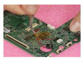
5. Remove 2 screws (M2\*3L(K)) and disconnect the DC IN cable then take away the DC IN jack.
