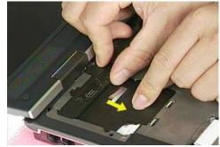
2. Disconnect 2 antenna cables, then open two latches to pop up wireless LAN module at 45 degrees angle and pull it out.
