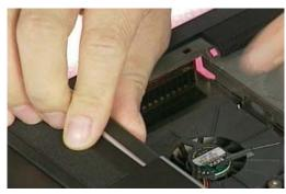
2. Remove 2 screws (M2.5\*6L(K)) at bottom case.
