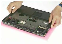
4. Disconnect touch pad FPC cable and remove 6 screws(M2\*3L(K)) then take touch pad backet off and take touch pad away.
