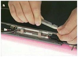
5. Remove 8 screws(M2.5\*6L(K)) and 2 fixed slices off , then take the LCD Bracket away.
