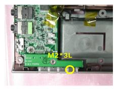
2. Remove 7 screws (M2\*3L(K)) and 2 tapes then disconnect modem cable then take the modem board.
