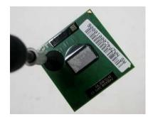
Note: If thermal module has no thermal pad on it, please plus a thermal pad on the CPU die before assembling.
