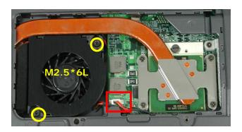
3. Remove the 4 screws (M2\*6L(K)) by order upon the thermal module and take away the CPU heat sink module gently
