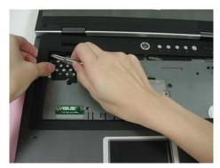
4. Loosen the switch board cable and take the keyboard cover away , then remove the switch cable.
