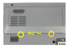
2. Remove 2 screws(M2.5\*6L(K)) and disconnect the FAN connector and then take away the Fan Module.
