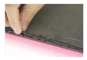
10. Remove 1 screw (M2.5\*4L(K)) and 1 screw on the other side, then take right and lift hinge off.
